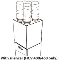
Connect ducts to the spigots on the silencer (The silencer is already fitted with spigots)
